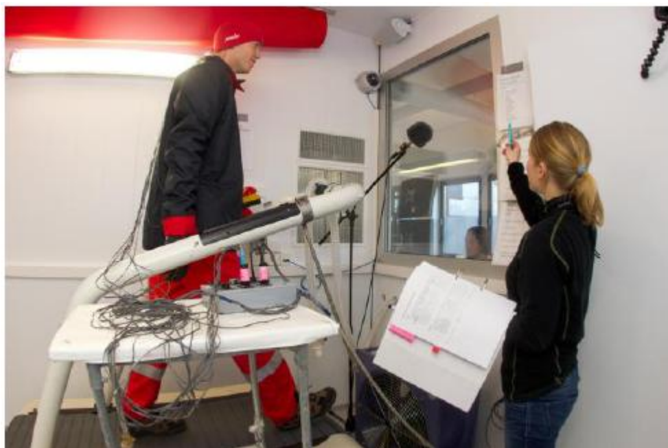
Figure 3. Work Physiology Laboratory SINTEF. Evaluation of a jacket with integrated PCM during activity cycles (walking period). The subject is voting his perceived thermal sensation and comfort, while skin and core temperatures are continuously monitored.
